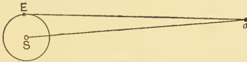
FIG. 91.—Diagram illustrating Parallax.
